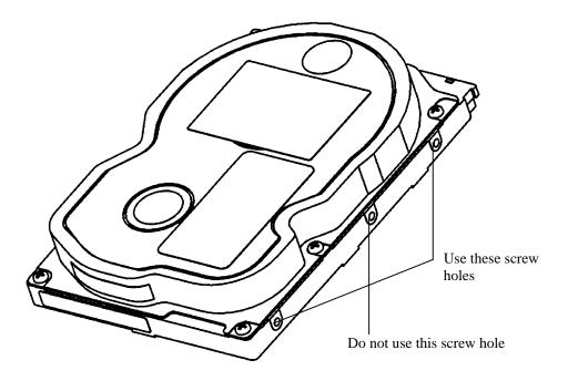
Figure 3.4 Limitation of side-mounting
